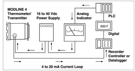
Modline 4 two-wire transmitter diagram
